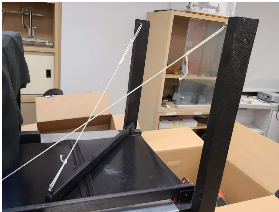
Figure 14: An image of the complete arm sorting system with the supporting strings connected to the rear vertical beams.
