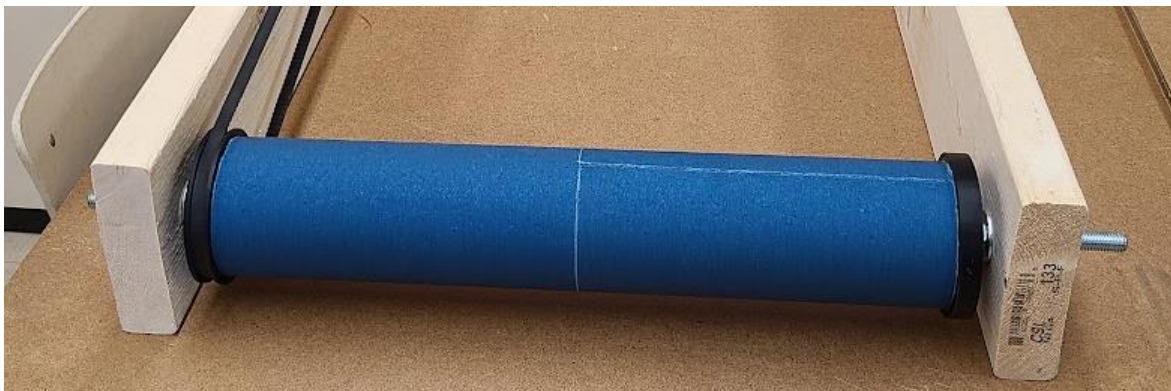
Figure 9: An image of the completed belt roller. The blue outer surface consisted of sandpaper and the caps were attached to the rollers via epoxy. The left side contains a specialized cap with a gear to turn the roller.
