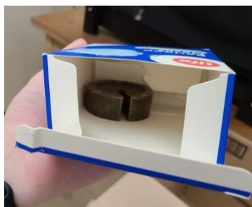
Figure 20: An image of the experimental object used to verify if the arms could distribute the required weight of 0.5 kg as required by the Success Criteria.
